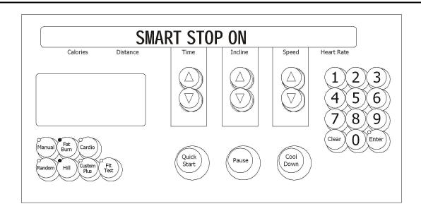
Upon entry into the test, if the smart stop PCB is not plugged in, a message will be displayed "Smart Stop Unplugged". This test will allow the user to test the Smart Stop System. If the smart stop system detects a user it will scroll the profile window from empty to full depending on the percentage of detection that is occurring. Other smart stop information will scroll automatically every 3 seconds.
